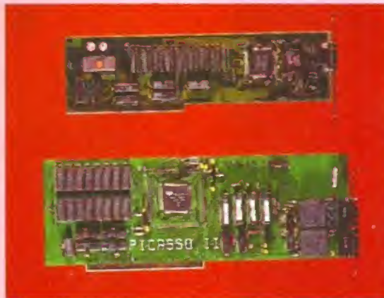
The Retina and Picasso cards are very good alternatives for the non-AGA set. A 256 colour Workbench can still be yours.
